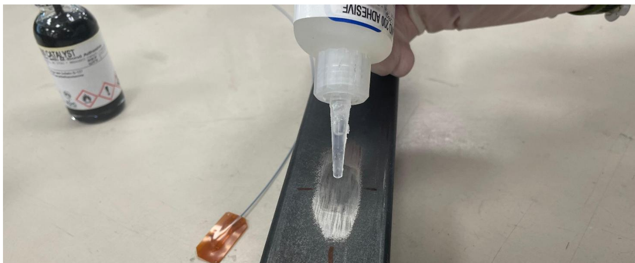
Figure 5: Application of the M-Bond 200 adhesive in the center of the area where the sensor should be placed.
