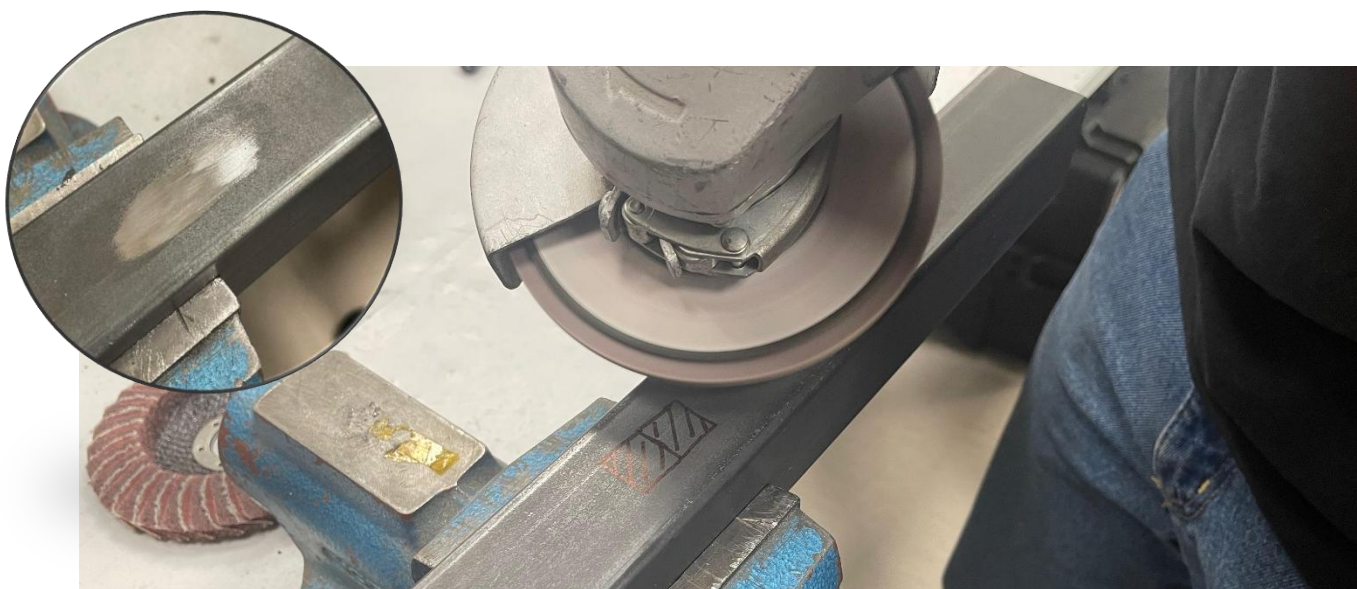
Figure 1: Mechanically cleaned area using an electrical grinding tool.
