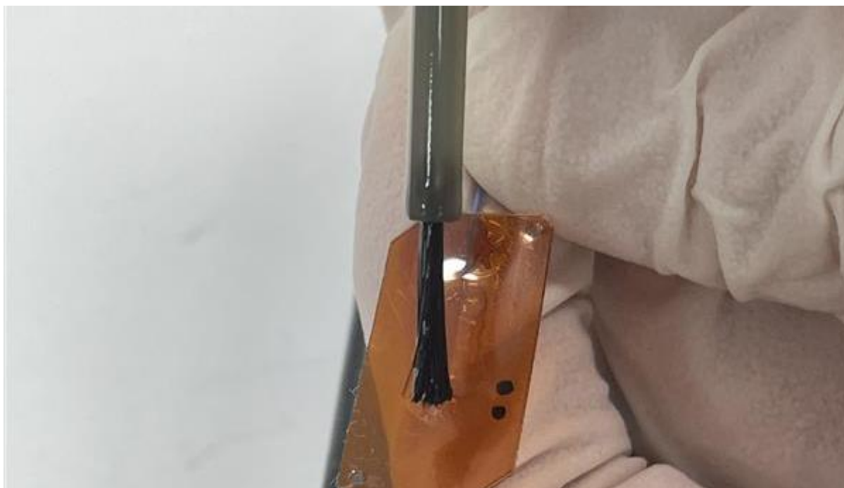
Figure 4: Application of the catalyst onto the bottom surface of the sensor using the appropriate brush.
