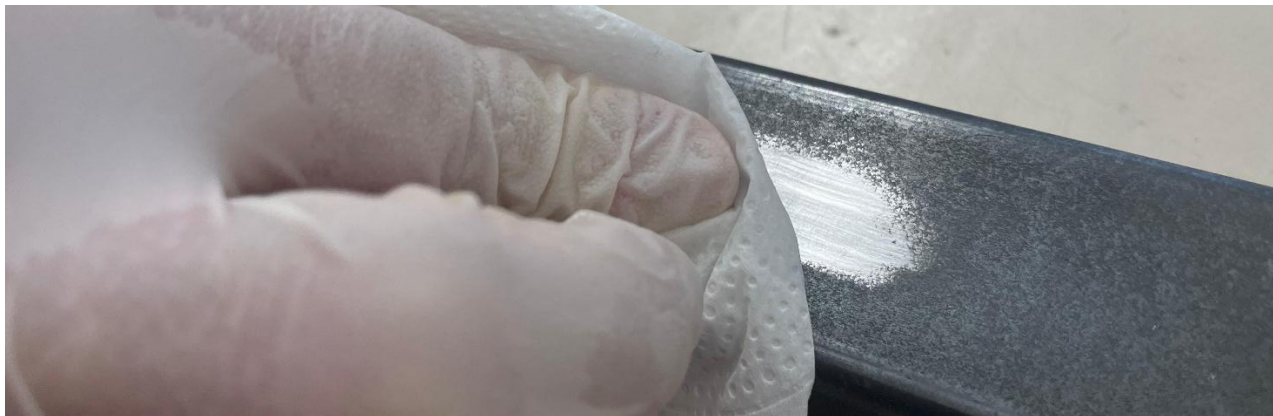
Figure 2: Degreasing and chemical cleaning of the surface.
