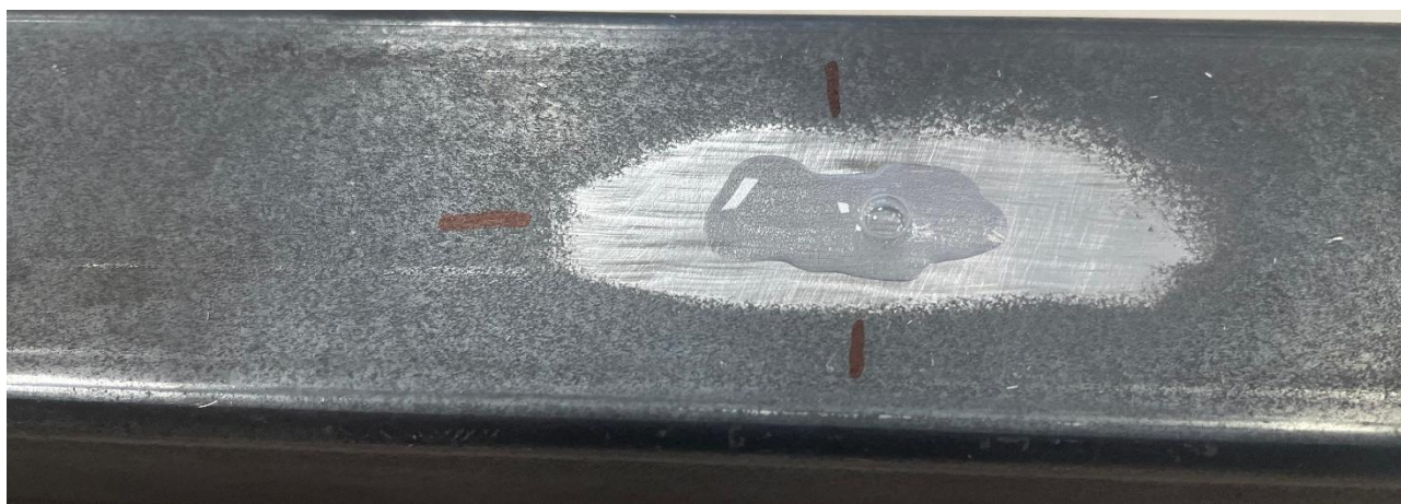
Figure 3: Chemical surface preparation by etching.
