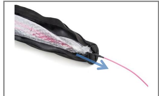
Insert the fanout section (protected by bubble foil) inside the Corpull. Be sure that the fabric of the Corpull encases the bubble foil on its entire length.
