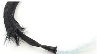
Remove insulation tape and plastic loop, then pull whole sleeve off.
