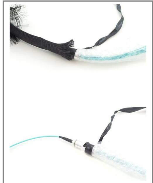
Remove bubble wrap by pulling towards end where bubble wrap is sealed.
