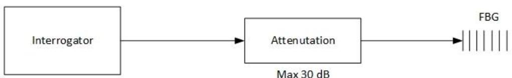
Figure 1: Max. allowed attenuation within optical line (bidirectional)
